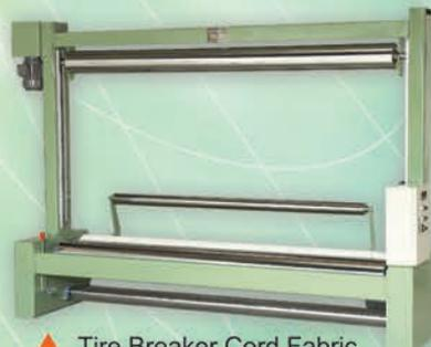
▲ Tire Breaker Cord Fabric Winding Machine
